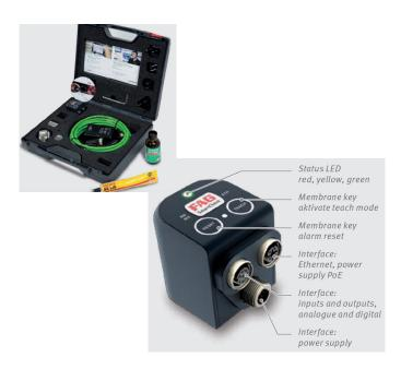
The FAG SmartCheck is a compact, modular, online measuring system for continuous, decentralized machinery and process parameter monitoring. Schaeffler offers a supplementary solution package, the FAG SmartCheck Service Kit, which is aimed specifically at users who already have initial experience of machine diagnosis.
