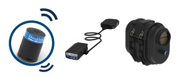
The Filter Minder® wireless monitoring system enables you to service your vehicle / equipment exactly when you need it. The Filter Minder wireless sensor makes use of the existing Geotab telematics infrastructure. Installation is easy — simply screw the sensor into the air cleaner indicator port and connect the receiver into the IOx port on the Geotab gateway.
