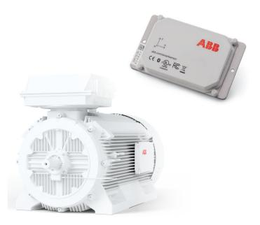
ABB Ability<sup>TM</sup> Smart Sensor for motors transforms simple motors into intelligent machines that tell you when they need servicing. Smart sensors are remote condition monitoring devices that attach to the frame of the motor. They provide information on operating and condition parameters, such as vibration, temperature, overload and bearing condition. The data is analyzed by a specifically developed software program and provided to the plant operator for maintenance planning.
